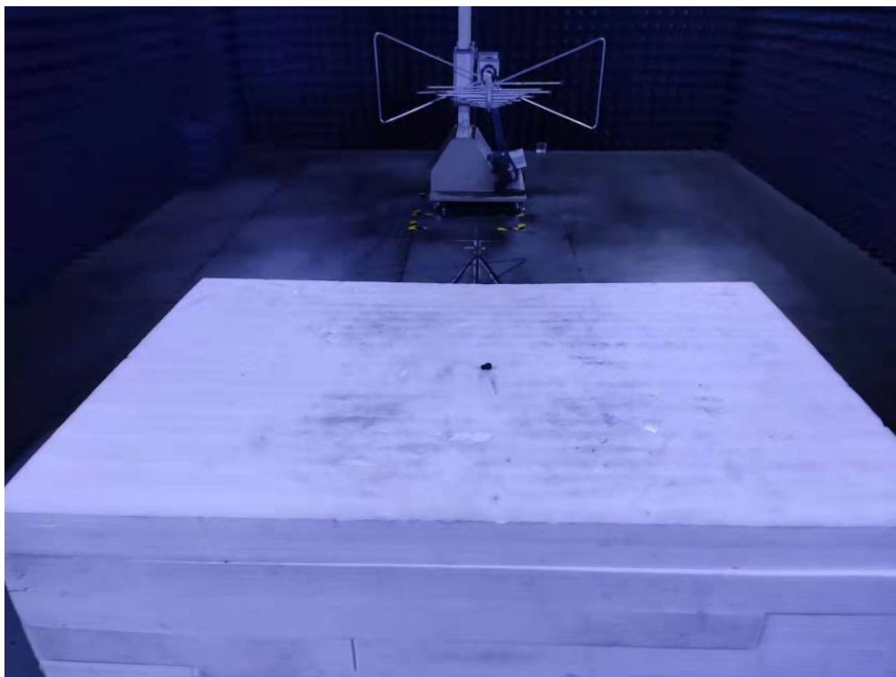
Photo of Radiated Emission Measurement (Below 1G)
