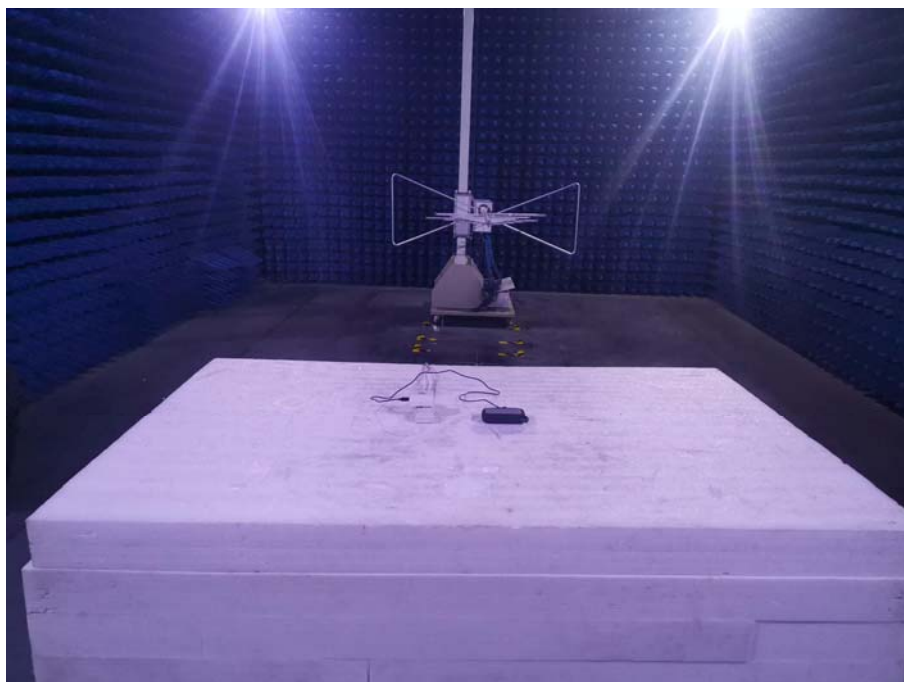
Photo of Radiated Emission Measurement (Above 1G)
