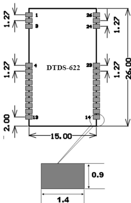
**Figure 3-** Physical Dimensions of the DTDS-622 Module (all units are in mm)
