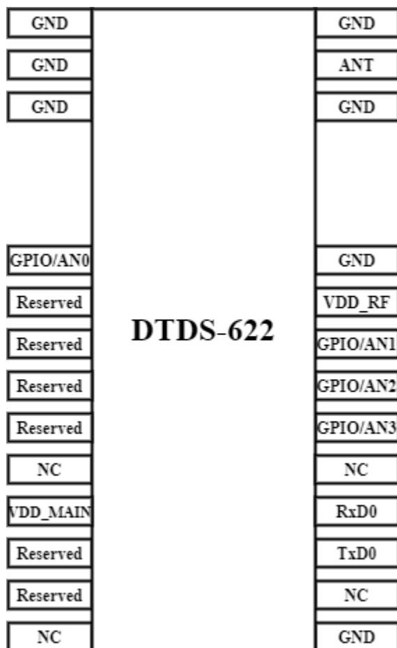
**Figure 1**- Top View of DTDS-622 Module
