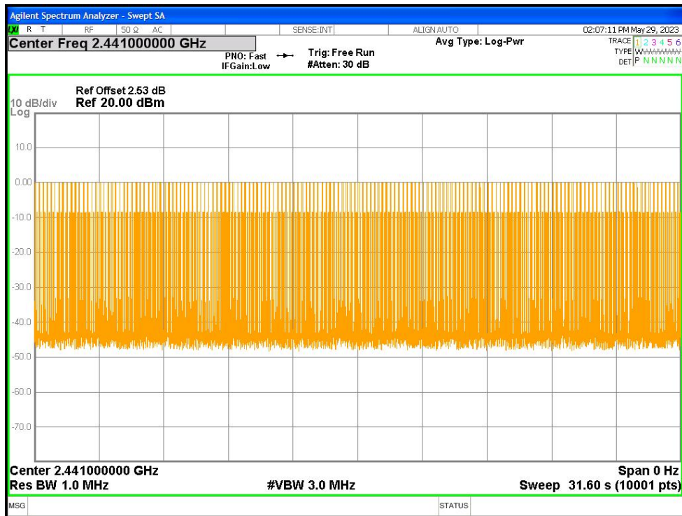
Dwell NVNT 1-DH3 2441MHz Ant1 One Burst
