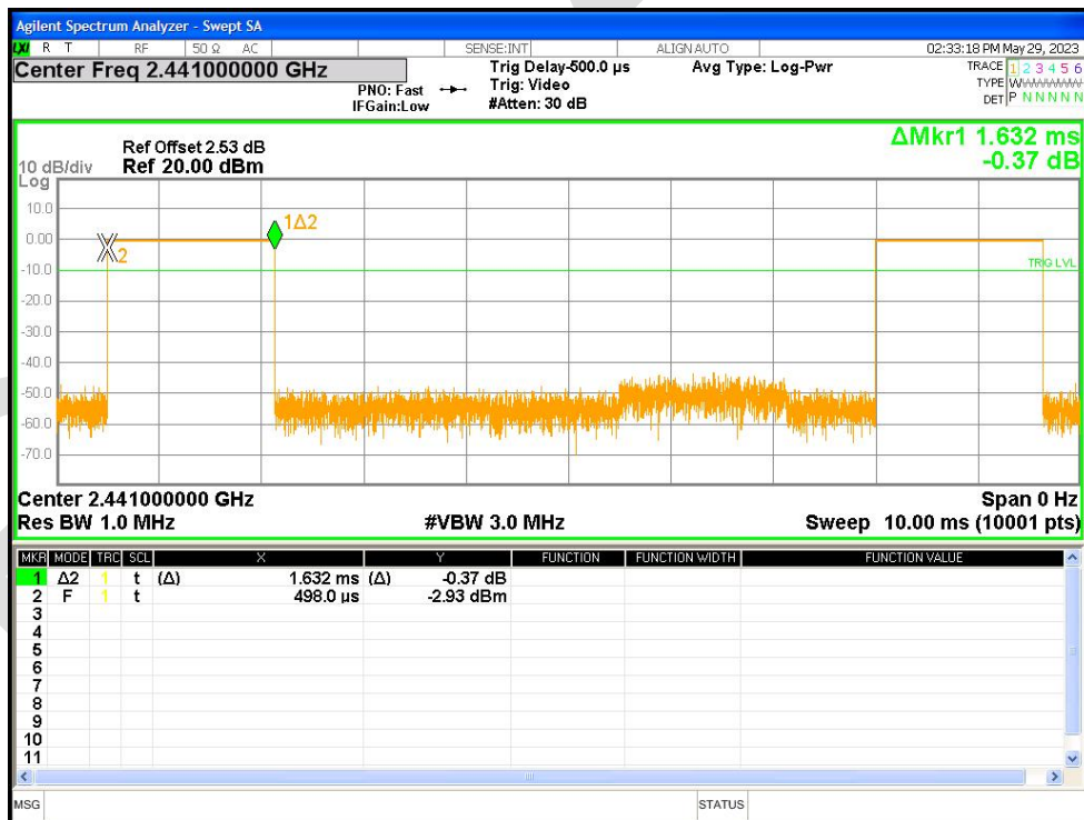
Dwell NVNT 1-DH3 2441MHz Ant1 Accumulated
