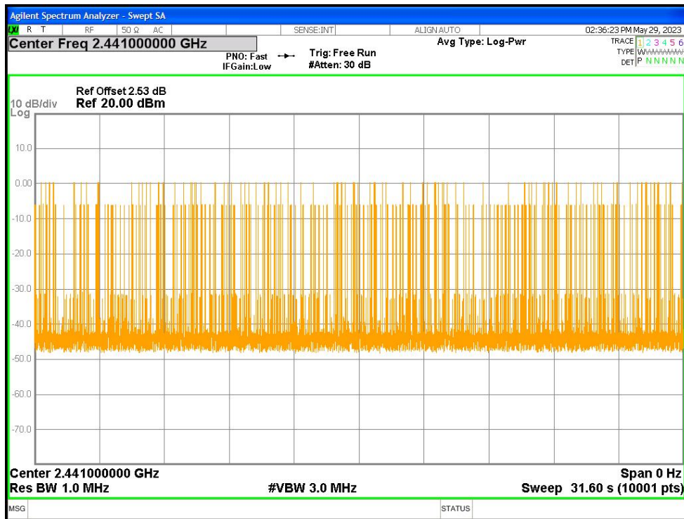
Dwell NVNT 3-DH5 2441MHz Ant1 One Burst
