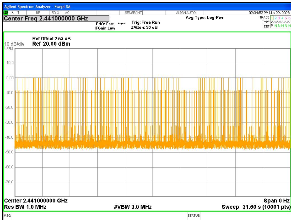
Dwell NVNT 2-DH5 2441MHz Ant1 One Burst
