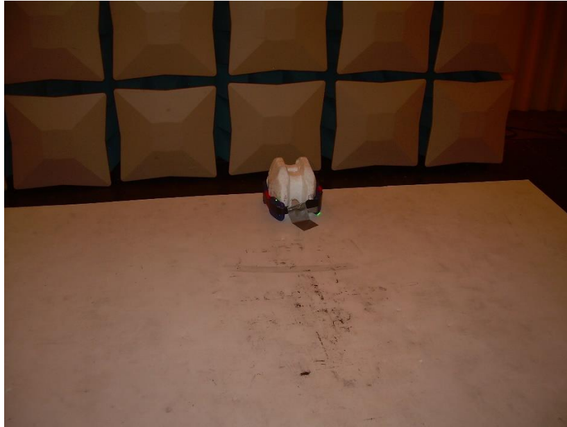
Photograph 1: Front View Radiated Emissions Configuration – Below 1000 MHz
