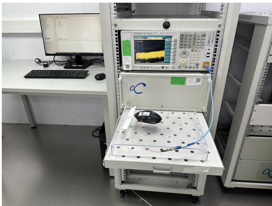
Conducted Test-2.4G ISM Band
