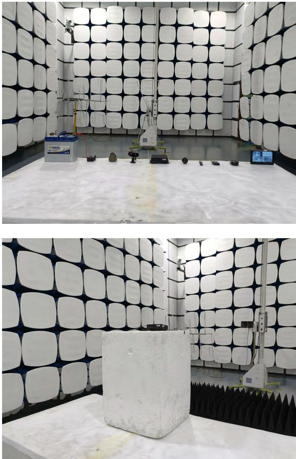
12.2.Photo of Conducted Emission test
