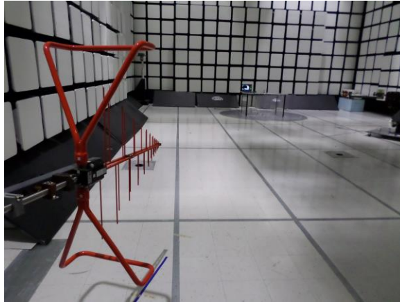
Figure 69: Radiated Spurious Emissions, 30MHz-1000MHz - Setup Antenna View
