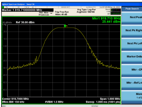
Peak output Power plot on channel 49
