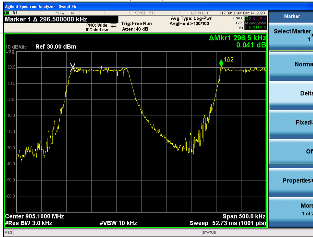
Channel Separation plot on channel 00-01
