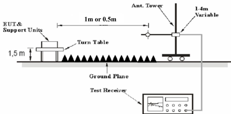
The antenna is scanned around the entire perimeter surface of the EUT, in both horizontal and vertical polarizations, at the distance of 1.0 m from 40 GHz to 90 GHz, and 0.5 m for above 90 GHz.
