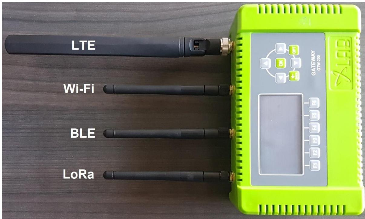
The GTW-200 is supplied with four antennas. Only the supplied antennas are approved for use.
