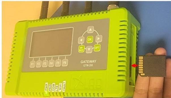
3. When the gateway restarts, it will automatically start the upgrade process. Follow any further screen instructions if/when prompted. Upon completion, the gateway will automatically restart and operate with the new firmware image. The newly installed firmware version number can be verified on the 'Setup' screen.
