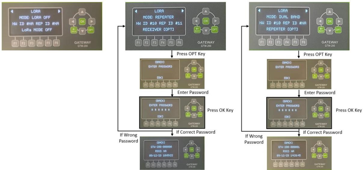
All submenus are password protected. The default password is [F1] [F2] [F1] [F2] [F1] [F2]. If the [BACK] key is pressed at any point while navigating in sub menu leads back to the upper menu (main menu) of that submenu.
