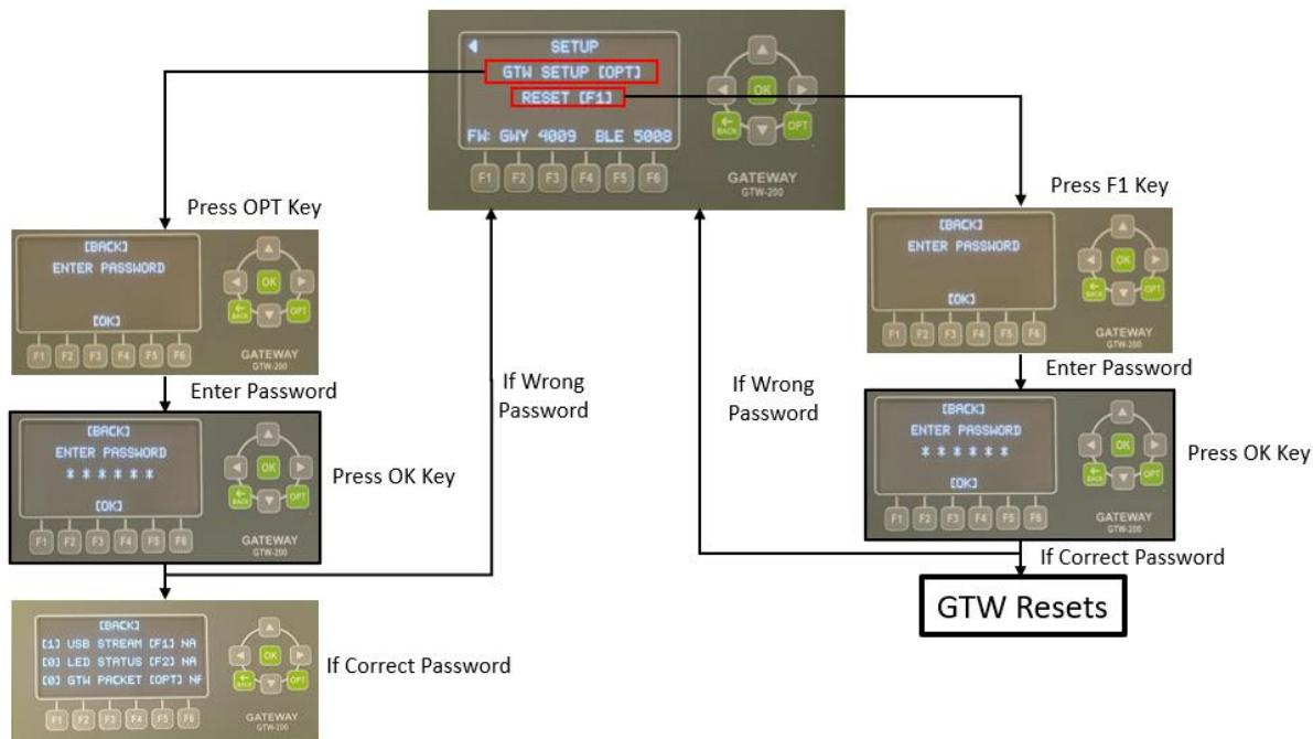
All submenus are password protected. The default password is [F1] [F2] [F1] [F2] [F1] [F2]. If the [BACK] key is pressed at any point while navigating in sub menu leads back to the upper menu (main menu) of that submenu.
