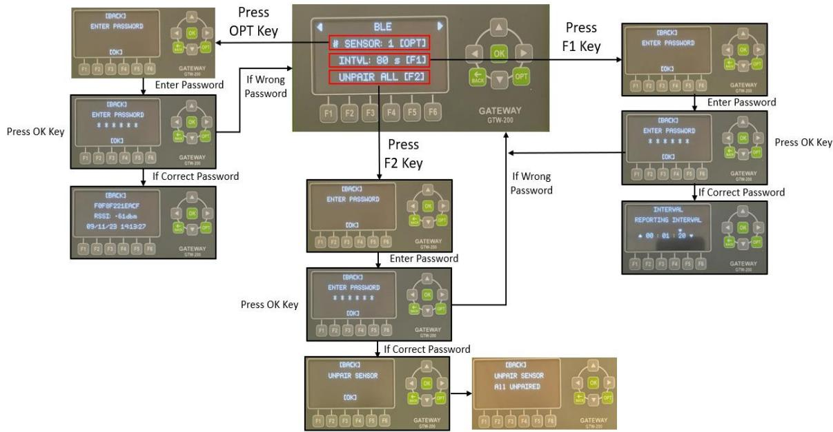
All submenus are password protected. The default password is [F1] [F2] [F1] [F2] [F1] [F2]. If the [BACK] key is pressed at any point while navigating in sub menu leads back to the upper menu (main menu) of that submenu.
