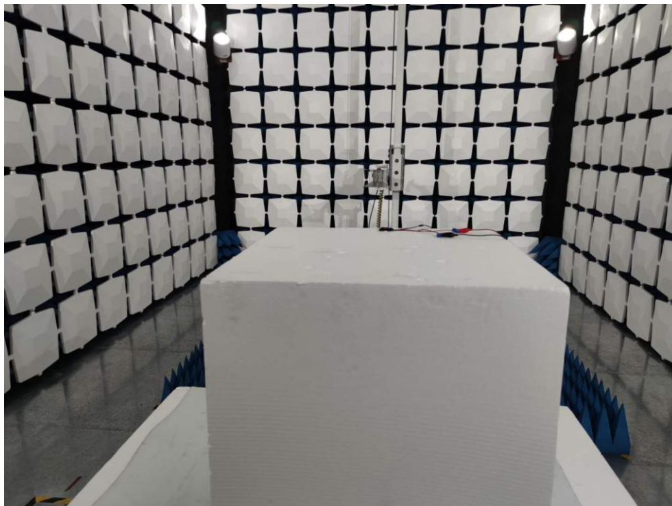
Above 1GHz for radiated emission test setup
