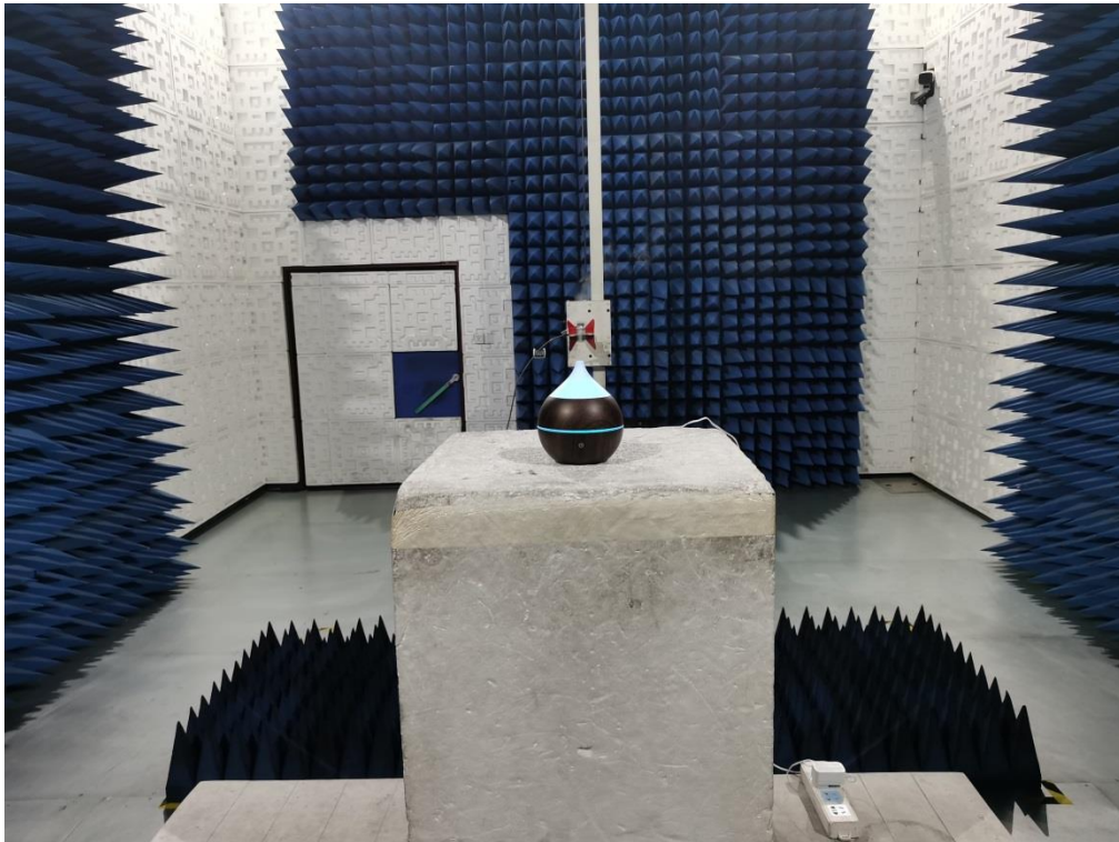
RADIATED EMISSION TEST SETUP ABOVE 1GHz
