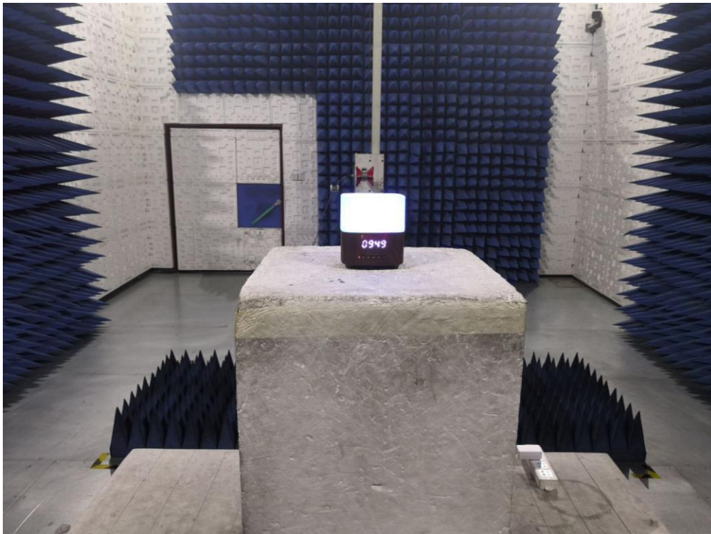
RADIATED EMISSION TEST SETUP ABOVE 1GHz
