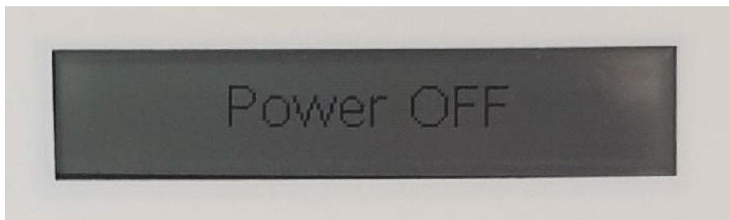
**When in this screen the device can be powered off by keeping pressed the button for more than 10 seconds.**
