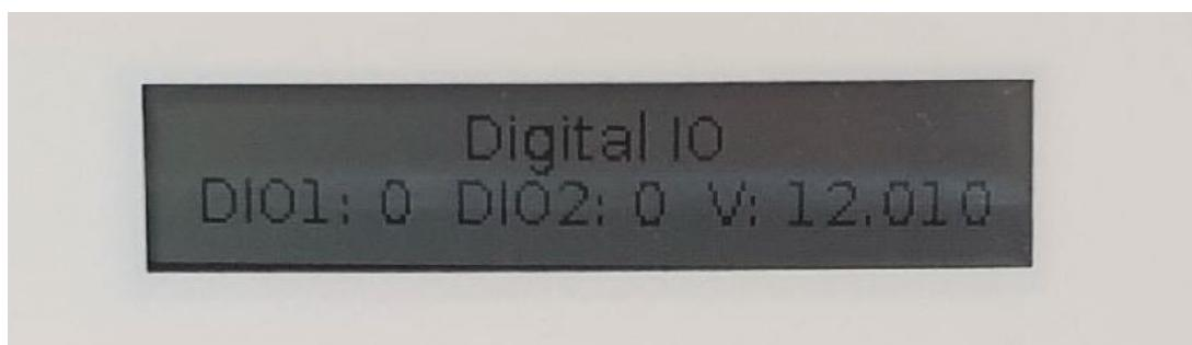
This screen is available only on device fitted with the Digital IO Expansion.
