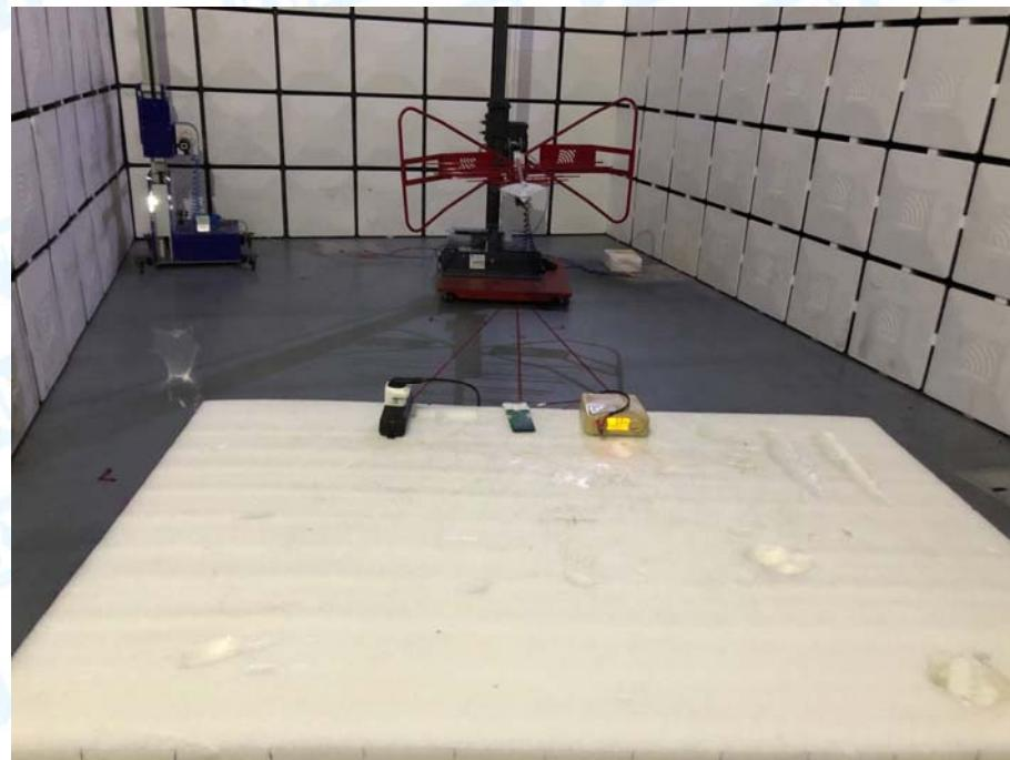
**Photo of Setup for Conducted Emission**
