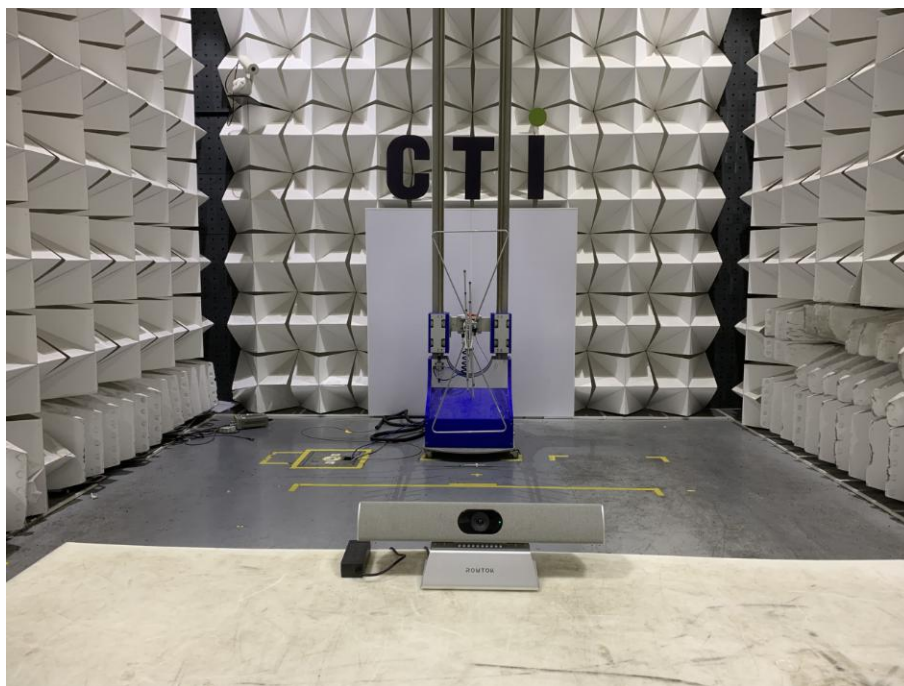
Radiated spurious emission Test Setup-1(Below 1GHz)
