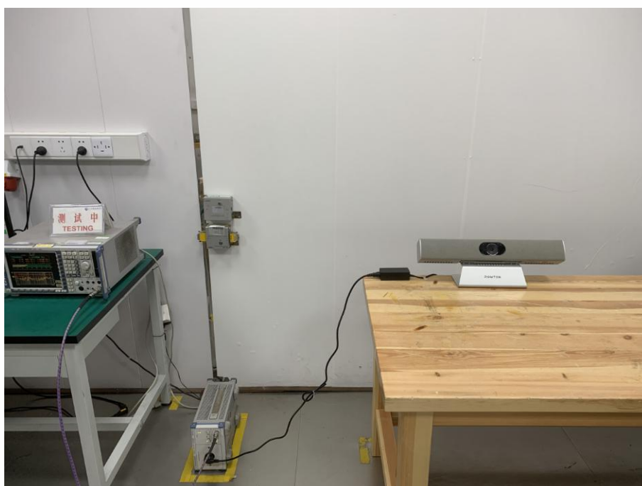
Conducted Emissions Test Setup
