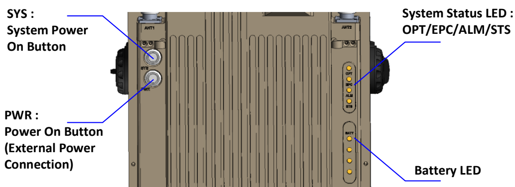
Figure 4. Power Switch and Status LED interface
