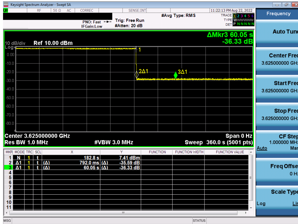
Plot 19. Conducted Measurement - RF transmission stops within transmitExpireTime + 60s. The last SAS heartbeat message is indicated by Marker 1 (X) (WINNF.FT.C.HBT.10)
