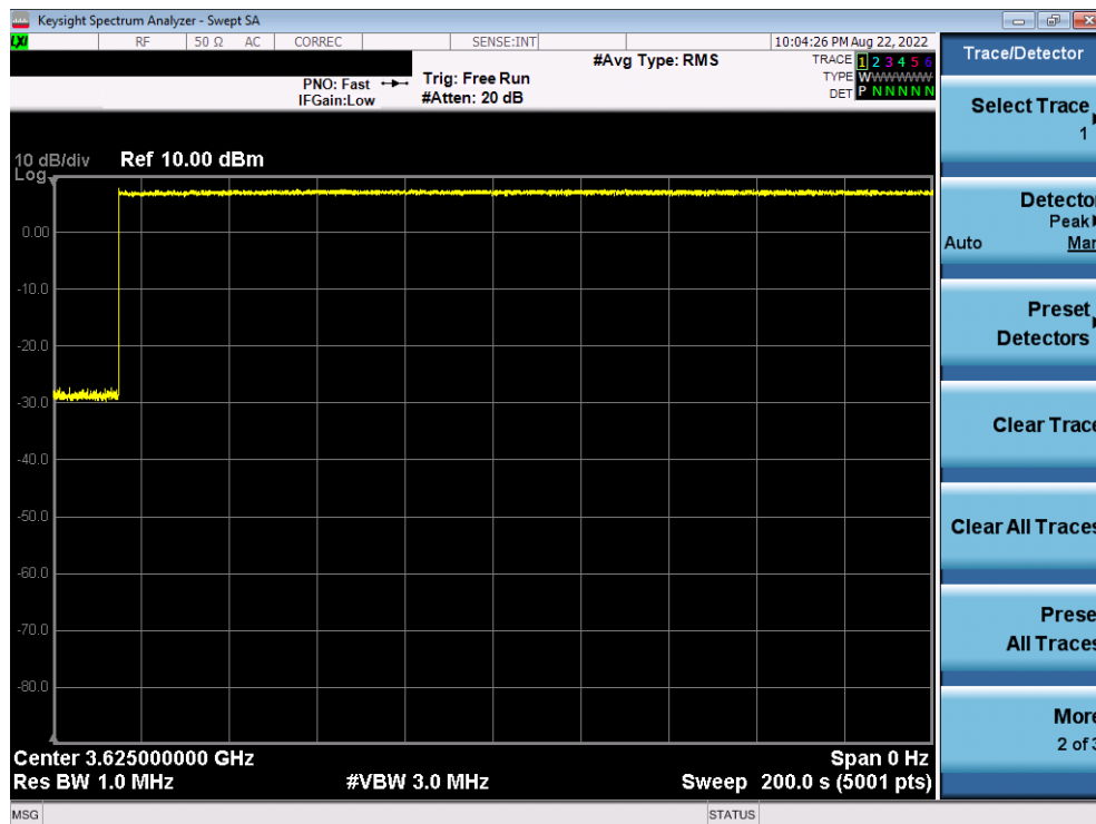
Plot 11. Conducted Measurement - RF transmission after SAS heartbeat response (WINNF.FT.C.HBT.1)
