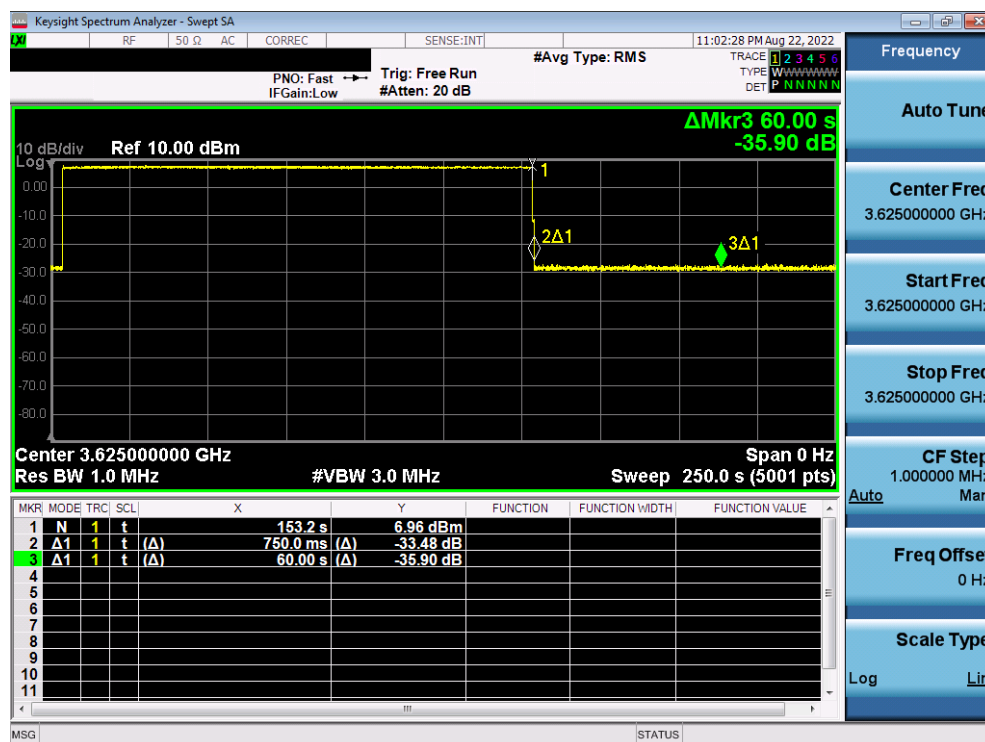
Plot 17. Conducted Measurement - RF transmission stops within 60s of SAS message. The SAS message is indicated by Marker 1 (X) (WINNF.FT.C.HBT.7)
