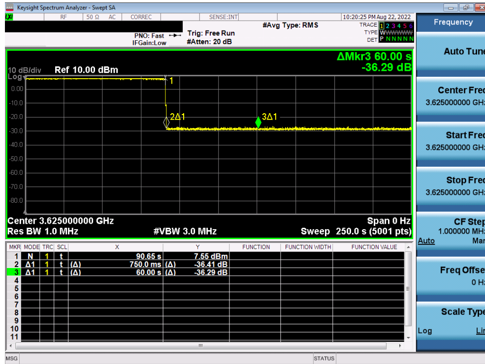
Plot 14. Conducted Measurement - RF transmission stops within 60s of SAS message indicated by Marker 1 (X) (WINNF.FT.C.HBT.4)
