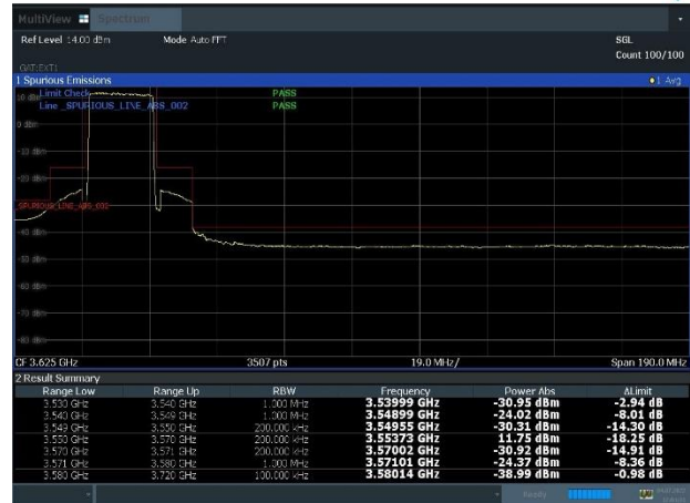
Plot 8-19. Channel Edge Emission Plot (LTE_B48_20M_QPSK – Low Channel, Port 1)
