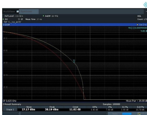
Plot 8-16. Peak To Average Power Ratio Plot (LTE_B48_10M_16QAM - Mid Channel, Port 0)
