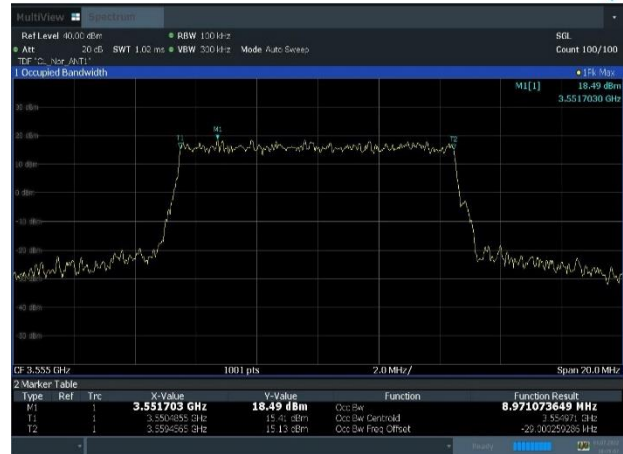
Plot 8-2. Occupied Bandwidth Plot (LTE_B48_10M_16QAM - Low Channel, Port 1)
