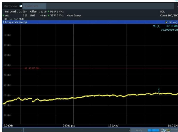
Plot 8-26. Conducted Spurious Emission Plot 6 GHz to 18 GHz (LTE_B48_20M_64QAM - Low Channel, Port 1)
