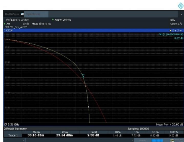
Plot 8-17. Peak To Average Power Ratio Plot (LTE_B48_20M_QPSK - Low Channel, Port 0)
