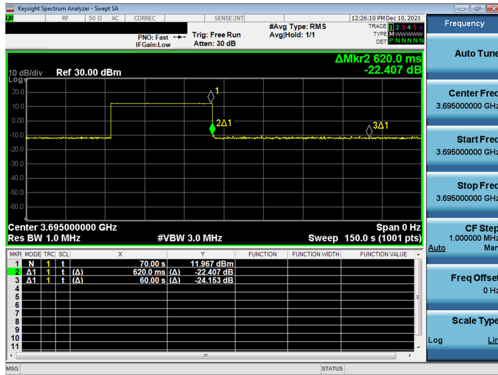
Plot 21. Conducted Measurement - RF transmission stops within 60s. The SAS message is indicated by Marker 1 (X) (WINNF.FT.C.DRG.1)
