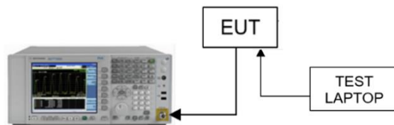
Figure 8-6. Test Instrument & Measurement Setup
