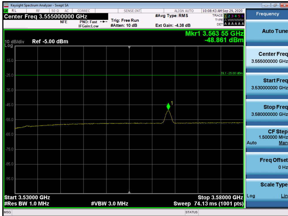
Plot 7-82. Conducted Spurious Emission Plot (10 MHz BW, Middle Channel, Port 0, 3530 MHz to 3580 MHz)
