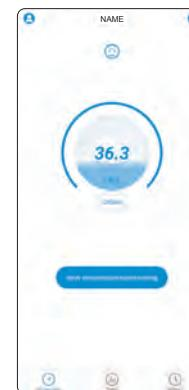
5. Click "Trend Graph", the interface will display your measured data in the form of graph(Can switch between Celsius and Fahrenheit)
