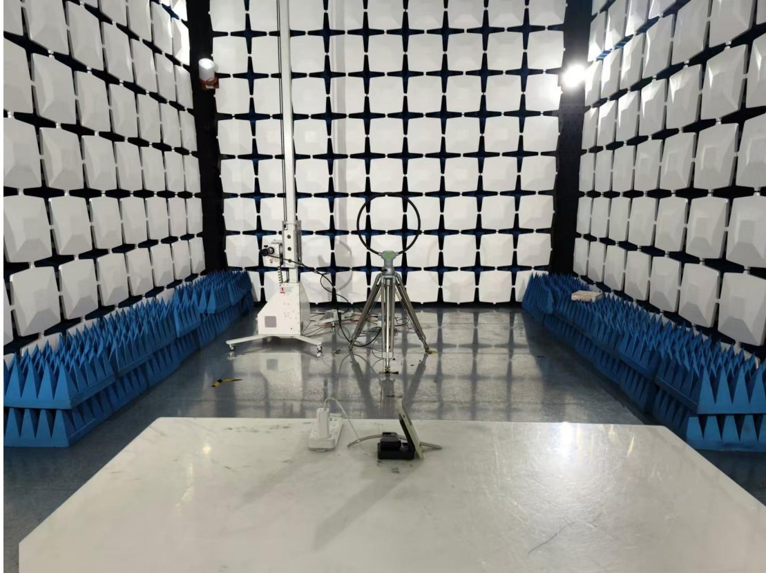
Blow 1GHz for radiated emission test setup
