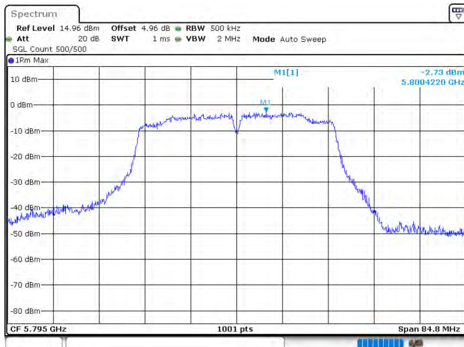
PSD NVNT 802.11n(HT40) 5795MHz Ant2
