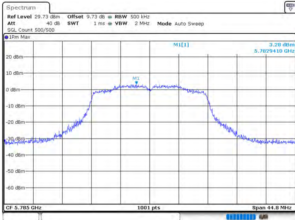
PSD NVNT 802.11n(HT20) 5785MHz Ant 2
