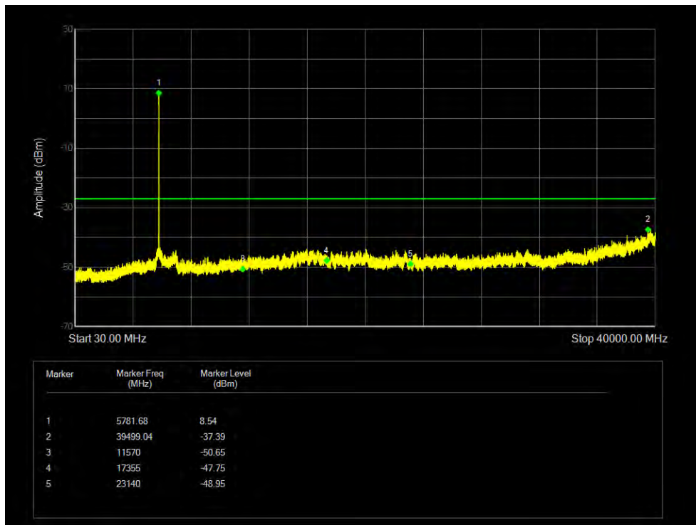
Tx. Spurious NVNT 802.11a 5825MHz Ant 2 Emission
