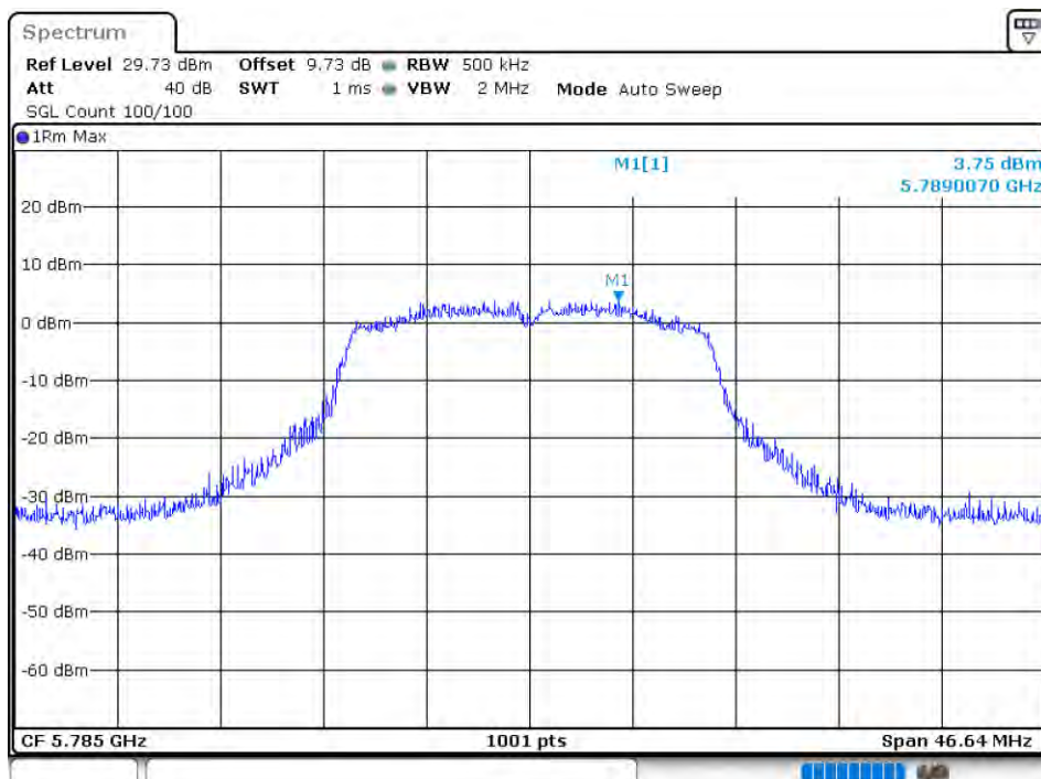
PSD NVNT 802.11a 5785MHz Ant 2
