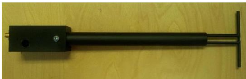
Figure 1 – MVG COMOSAR Validation Dipole
