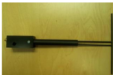
Figure 1 – MVG COMOSAR Validation Dipole
