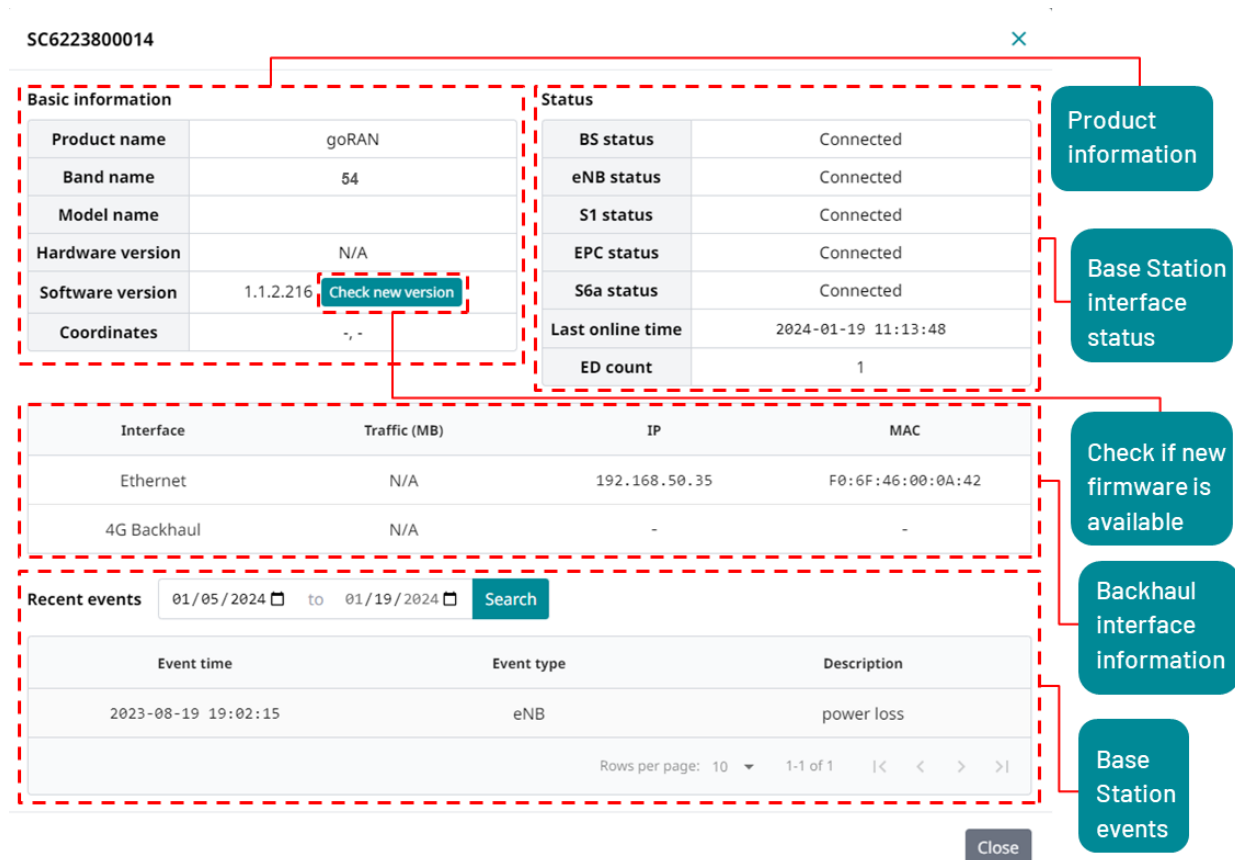
Figure 7.3.1-12 Base Station information
