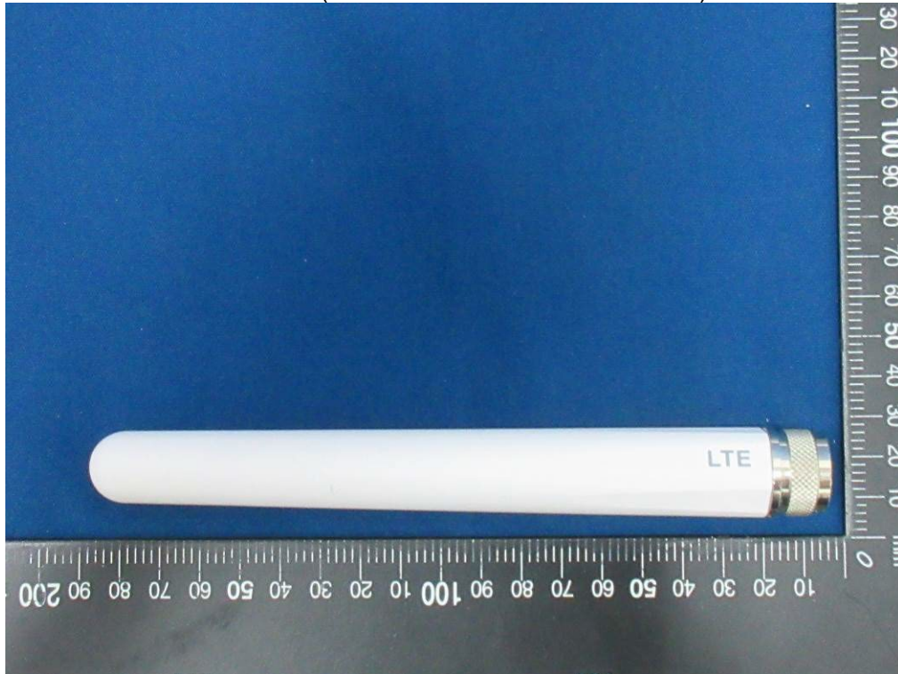
(28) EUT Photo - WWAN Antenna (Model No.: OA-LTEWB-035-C0-UB) for WWAN Module
