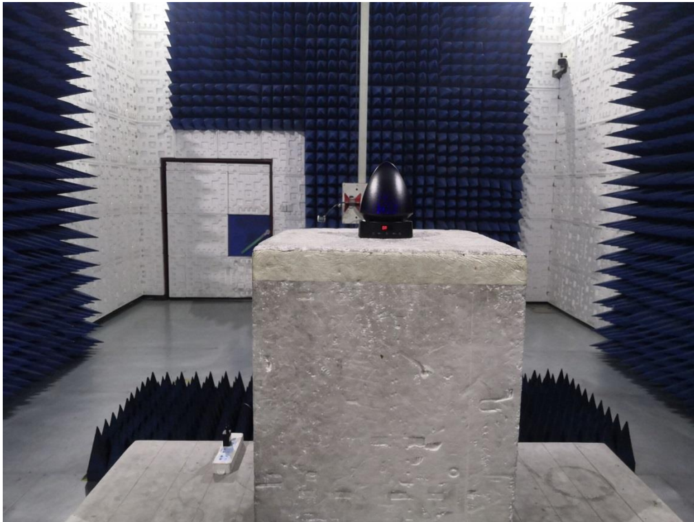
RADIATED EMISSION TEST SETUP ABOVE 1GHz
