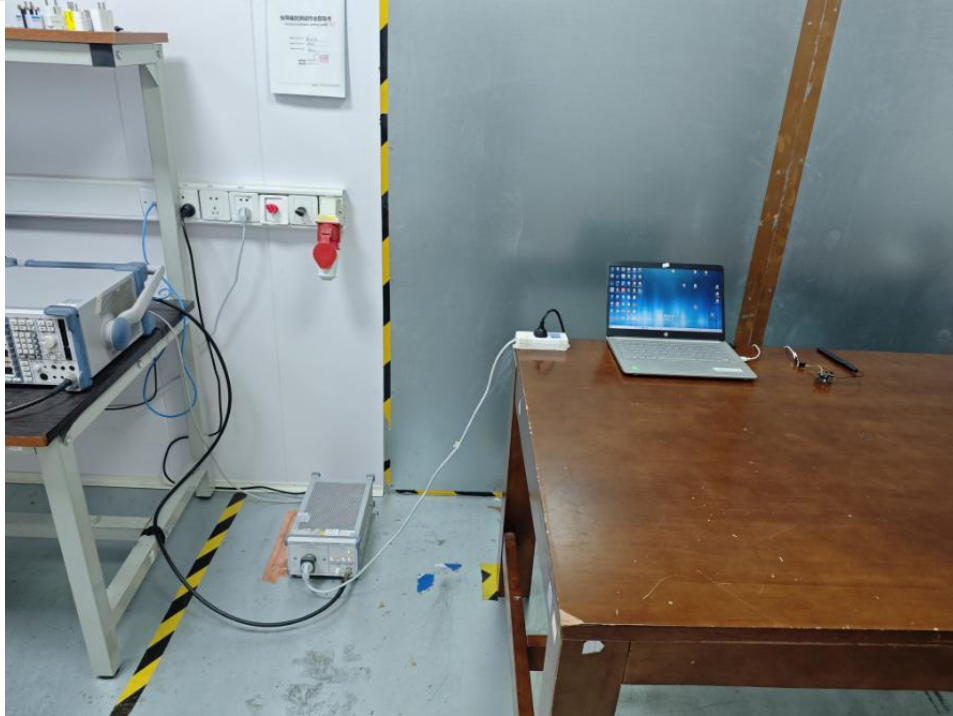
Conducted emissions at AC power line (150kHz-30MHz)
