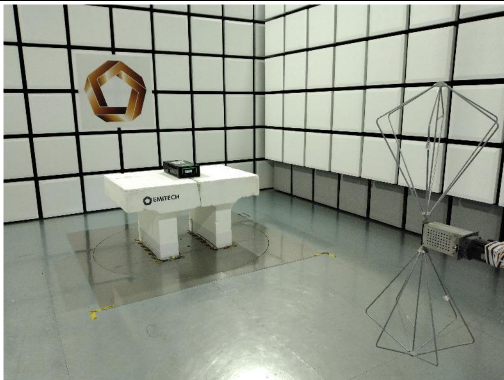
TEST SETUP PHOTO(S) - ICSD DN RM4V - SPURIOUS / LOW CHANNEL / P=-10 / F>1\text{GHz}
