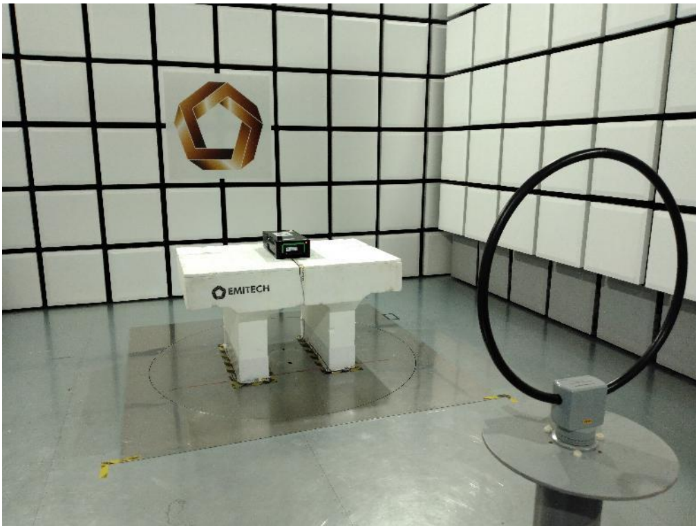
TEST SETUP PHOTO(S) - For F < 30\text{MHz}
