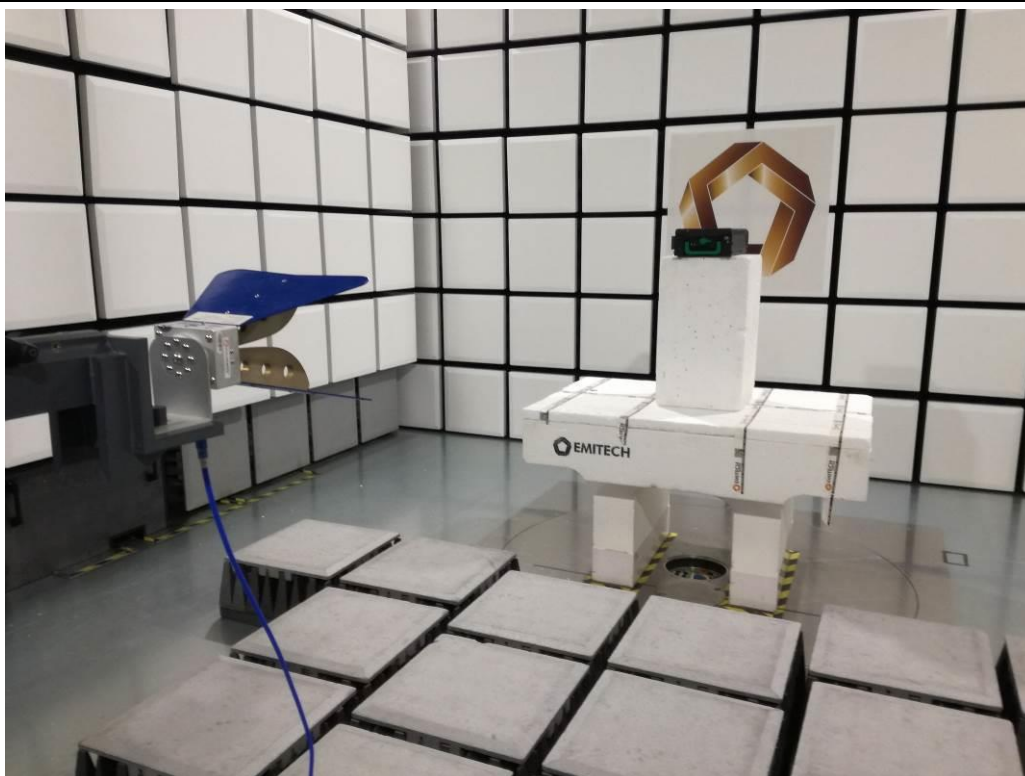
TEST SETUP PHOTO(S) - FOR FREQ > 1GHz
