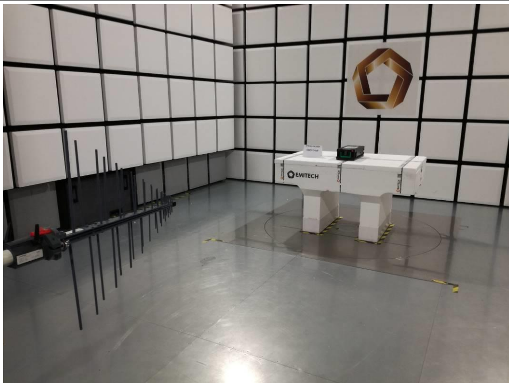
TEST SETUP PHOTO(S) - 200MHz < FOR FREQ < 1GHz
