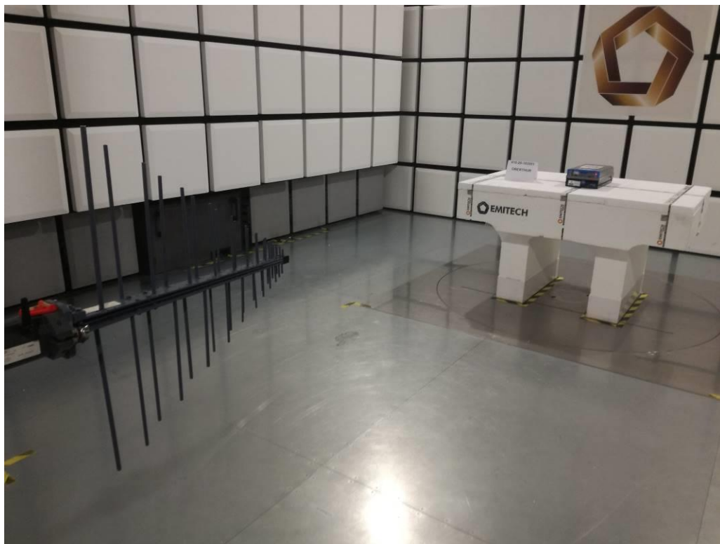
TEST SETUP PHOTO(S) - 200MHz < FOR FREQ < 1GHz
