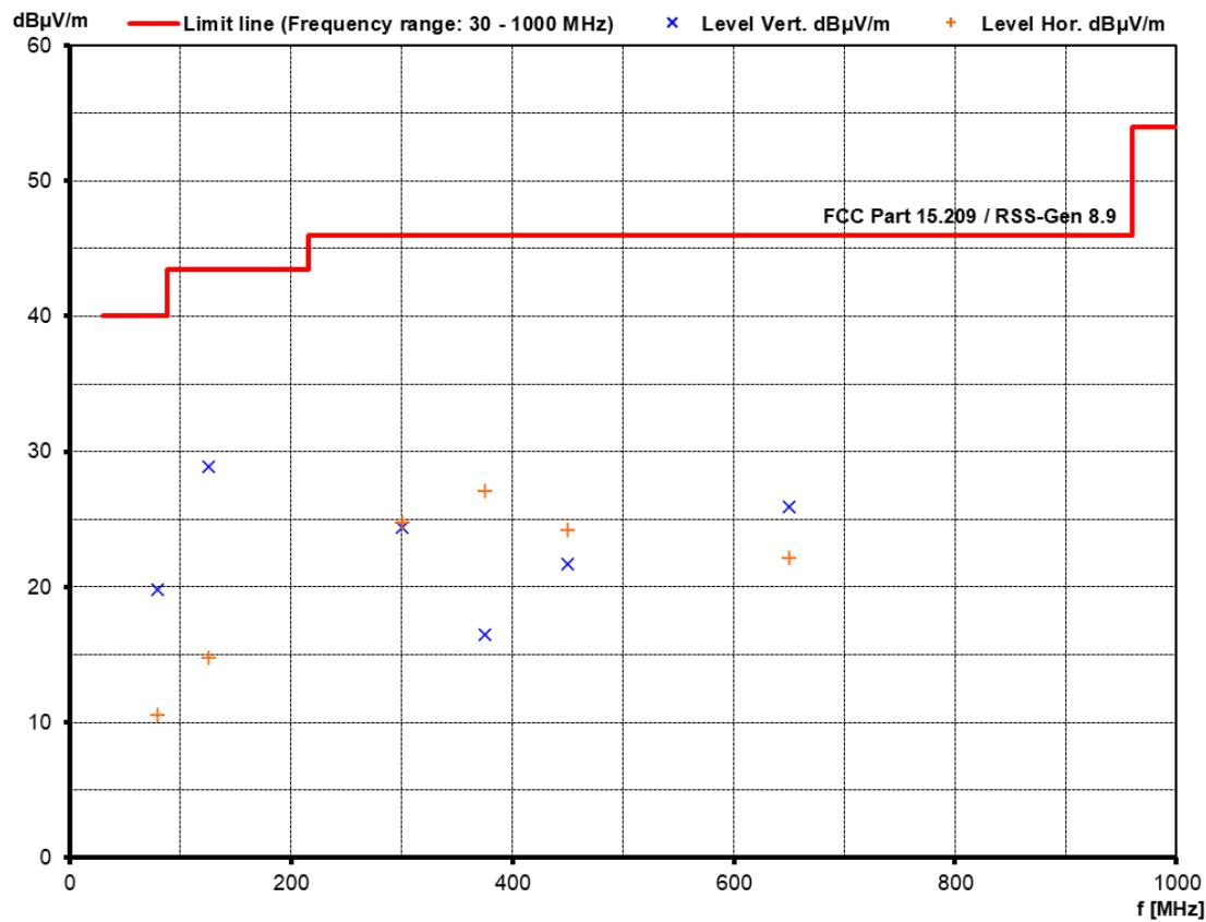
Note: For frequencies < 1 GHz the general radiated limit has been applied.
