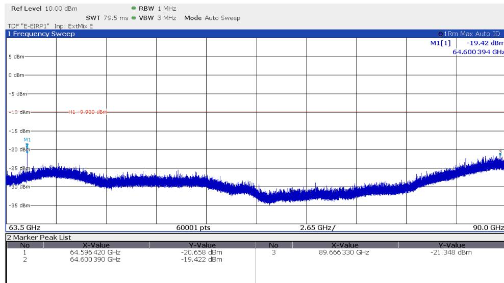
Note: To minimize unintended mixing products generated by the external mixer the AutoID function was used.
