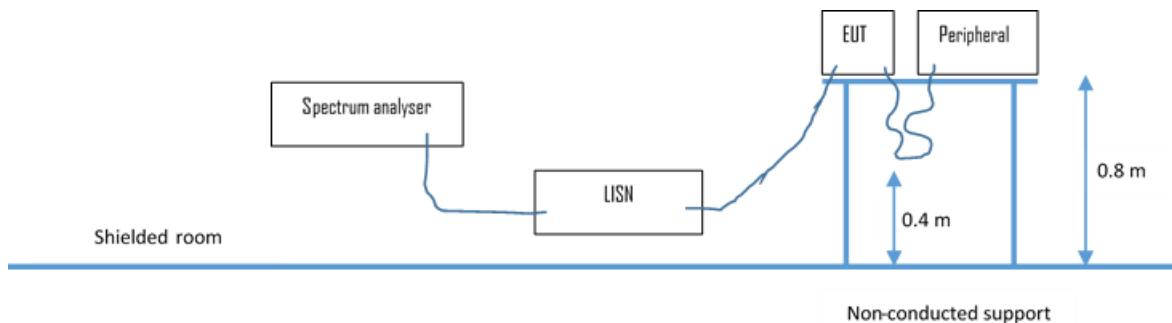
The final level, expressed in  $\text{dB}\mu\text{V}$ , is arrived at by taking the reading directly from the Spectrum analyser. This level is compared to the limit.
