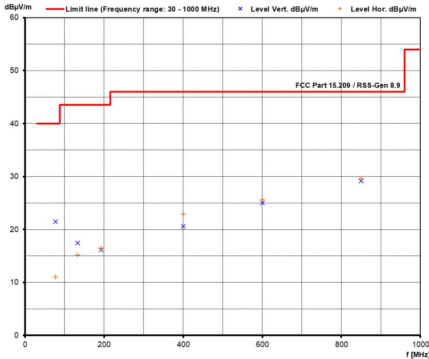
Note: For frequencies < 1 GHz the general radiated limit has been applied.
