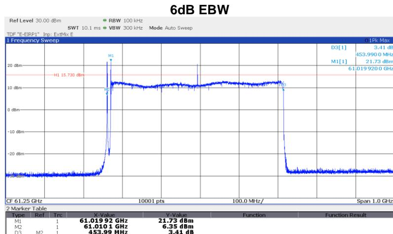
Note:  $f_{\text{high}}$  below 6dB reduction due to desensitisation of FMCW part for RBW = 100kHz, see below for  $f_{\text{high}}$  with RBW = 1 MHz, where no desensitization occurs.
