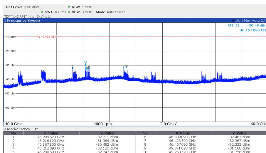
Note: To minimize unintended mixing products generated by the external mixer the AutoID function was used.
