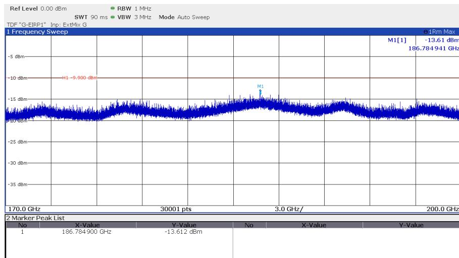
Average limit according to FCC Part 15C, Section 15.255(d):
