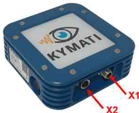
Figure 4.9: Bottom side X1 (DC connector) & X2 (Ethernet / PoE connector)
