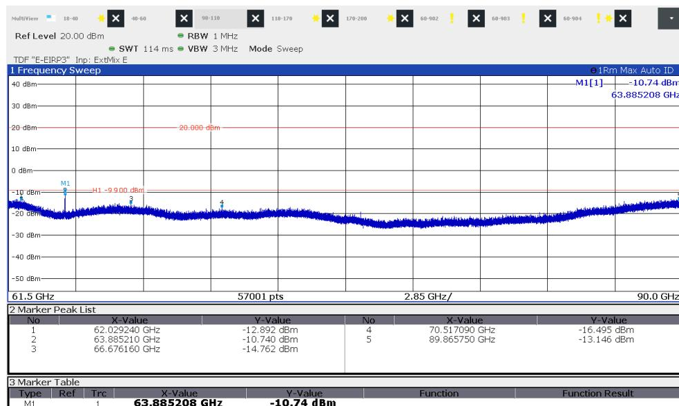
Note: The emission 63.885 GHz are caused by the external Mixer and is ignored.
