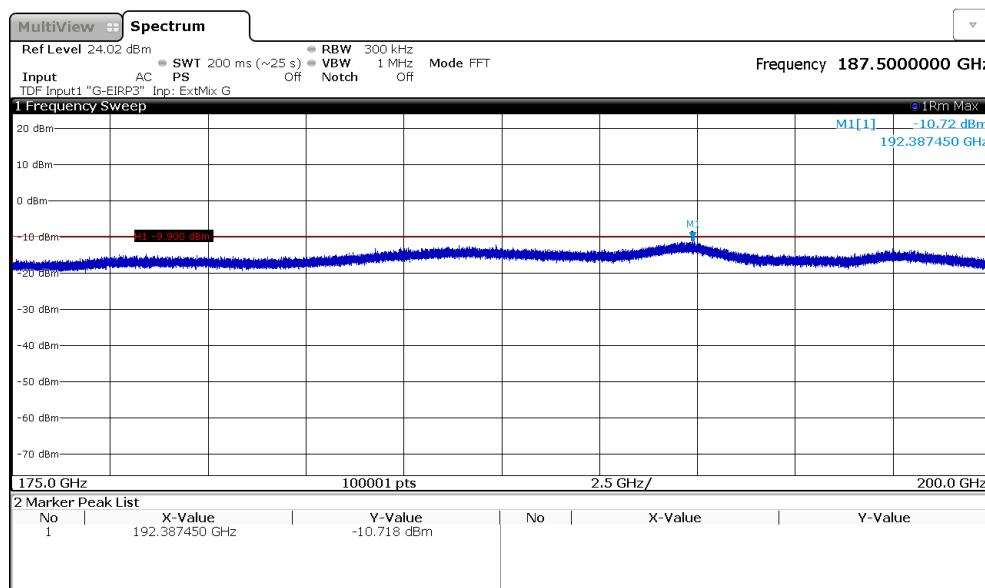
Note: This measurement is done with RBW=300 kHz in order to show no hidden emission is in the noise.
