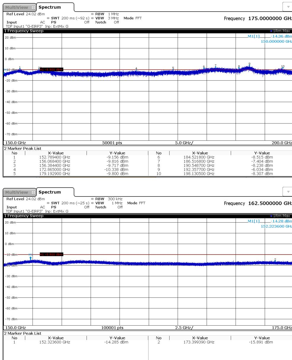
Note: This measurement is done with RBW=300 kHz in order to show no hidden emission is in the noise.
