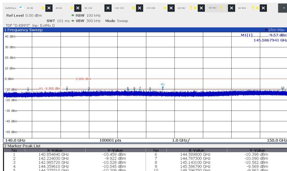
Note: This measurement is done with RBW=100 kHz in order to show no hidden emission is in the noise.
