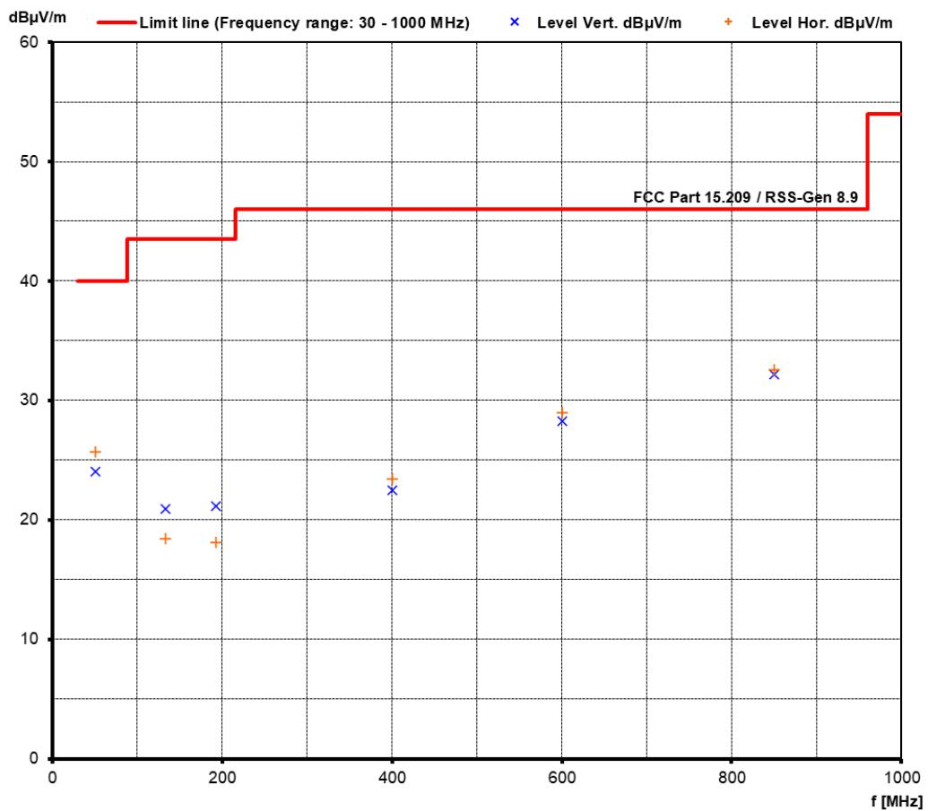
Note: For frequencies < 1 GHz the general radiated limit has been applied.
