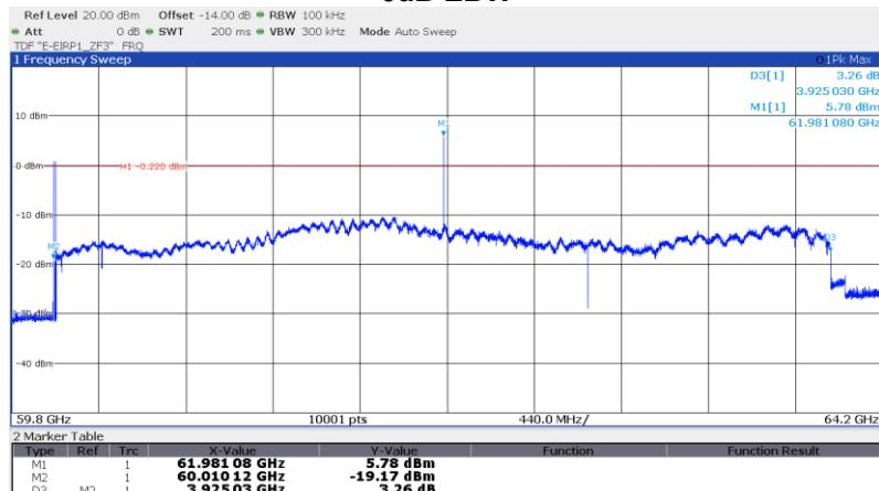
Note:  $f_{high}$  below 6dB reduction of FMCW part due to desensitisation for RBW = 100kHz, see below for  $f_{high}$  with RBW = 1 MHz, where no desensitization occurs.
