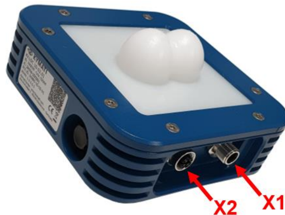
Figure 11: Bottom side X1 (DC connector) & X2 (Ethernet / PoE connector)
