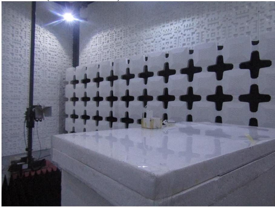
Conducted disturbance voltage at mains ports(150KHz-30MHz)
