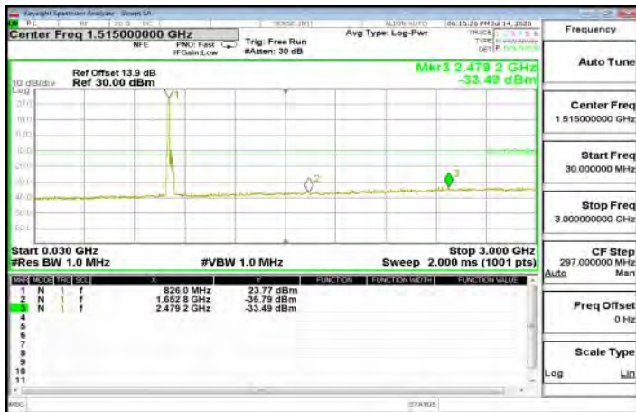
Spurious Emission Low_ HSUPA_B5_Mid CH4183-836.6
