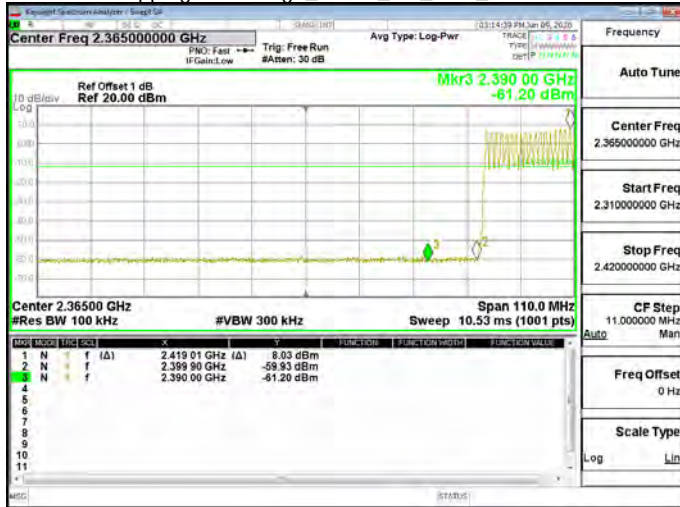
Hopping Band Edge_GFSK_1M_DH5_2402MHz
