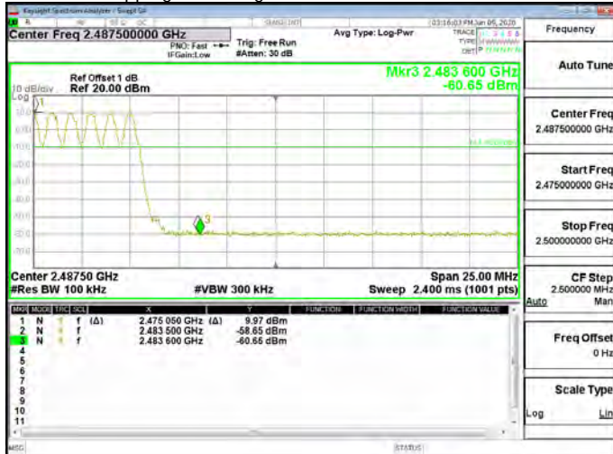
Hopping Band Edge_GFSK_1M_DH5_2480MHz
