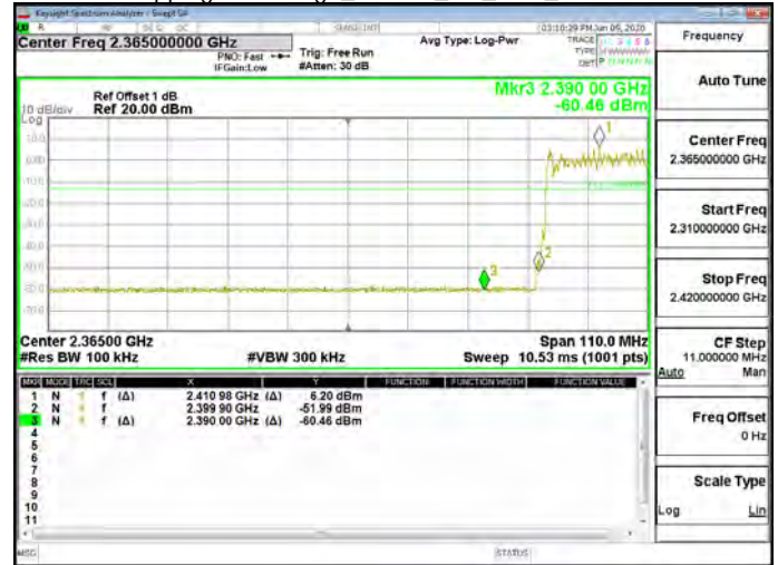
Hopping Band Edge_8DPSK_3M_DH5_2402MHz
