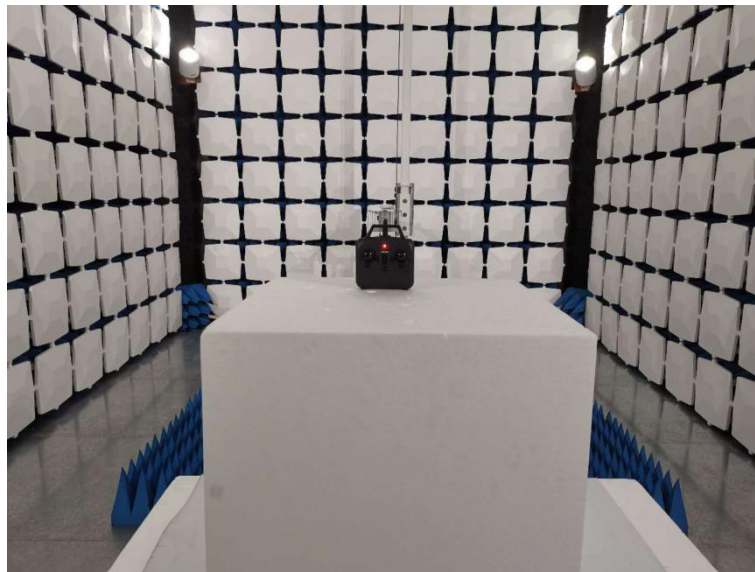
Above 1GHz for radiated emission test setup
