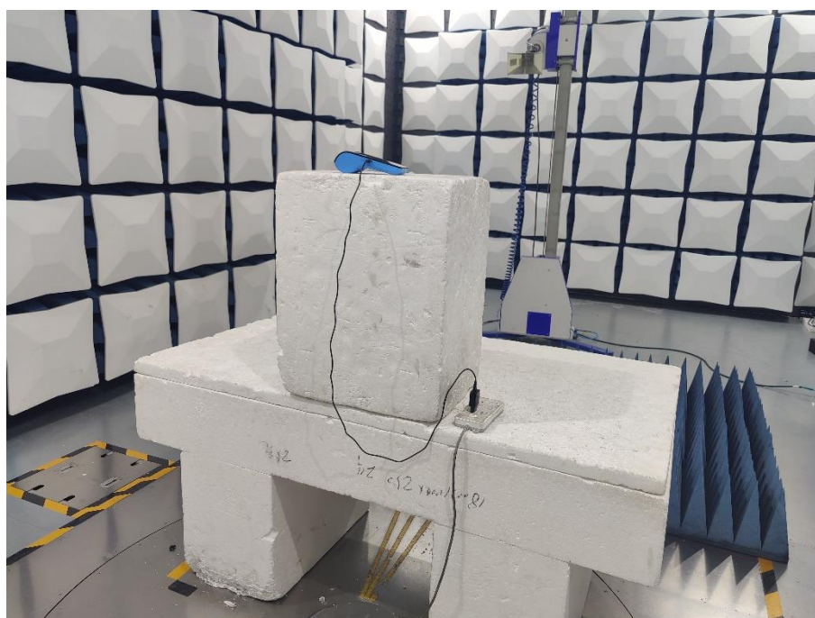
Radiated Emissions View (1GHz-18GHz)
