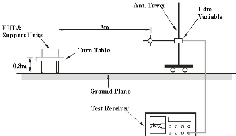
Note: Antenna is set up at 1m during test for below 30MHz.
