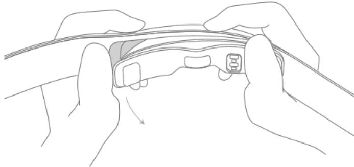
② Installation: Hold the main unit module squarely close to the headband cavity and automatically attach it (make sure the headband is oriented in the same direction as the main unit module).
