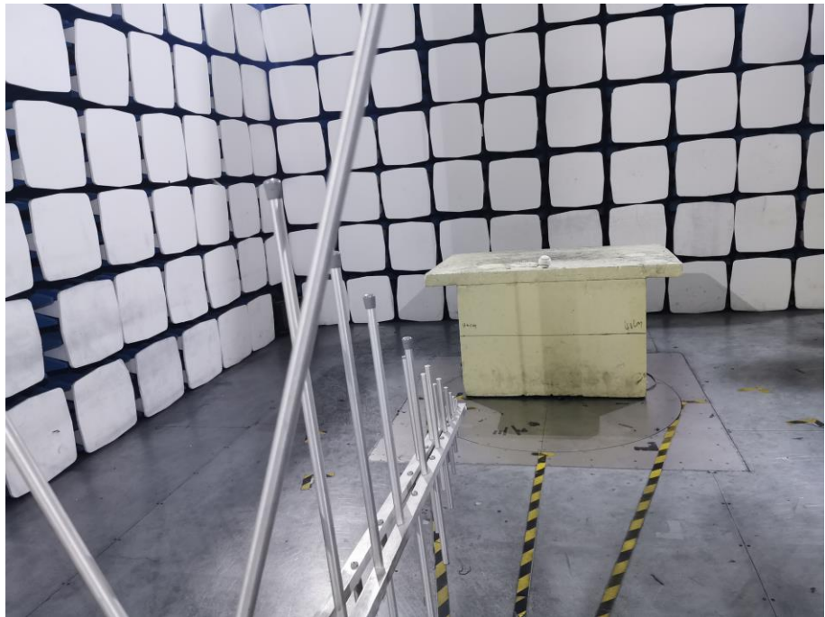
Radiation Emission Test Setup (30MHz to 1GHz)
